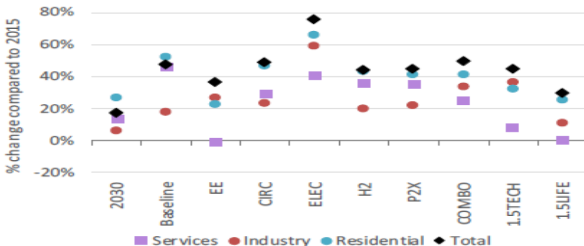
Figure 17: Changes in final electricity demand in EU28 for a range of scenarios, 2050 vs 2015 (%)
