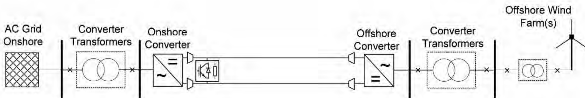
FIGURE 2.5: Onshore and Offshore Wind Power Plant Connection
