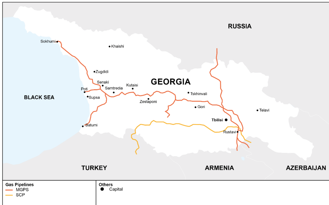
Figure 3.6 Georgia's natural gas pipeline network
